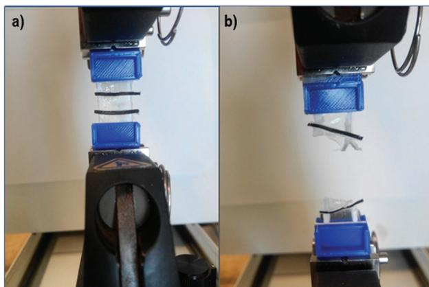
Figure 1. A sample glued between PLA grips and that fixed in the machine pneumatic system: a) at the beginning and b) at the end of traction test. Markers are visible on the sample surface.
