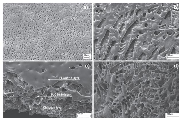
Figure 2. SEM micrographs a) one layered patch 1L, b) inner layer of two layered patch 2L, c) section of three layered patch 3L, and d) inner chitosan layer of patch 3L.
