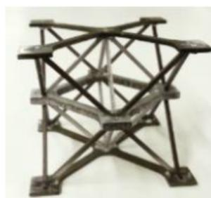
Bi-material building block with negative thermal expansion
