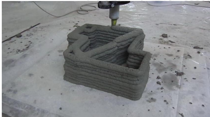
Phases of the 3d printing process of the beam segments.
