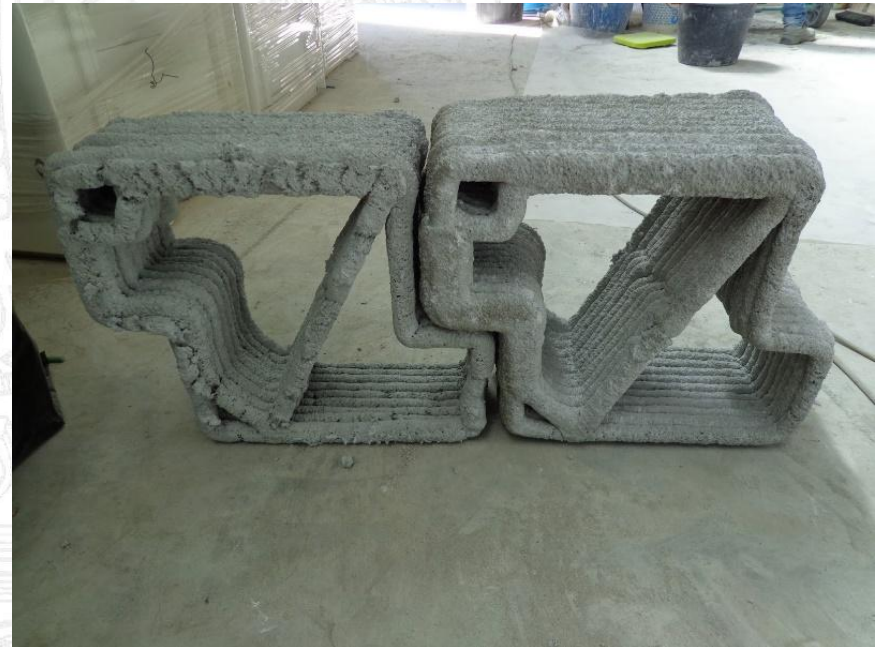
A number of holes needs to be designed to anchor the rebar.
